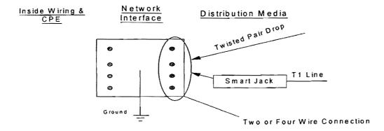
Figure 1 - Network Interface Device
