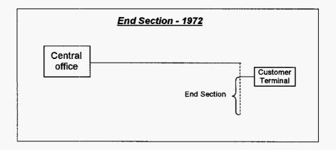
An end section should not be longer than 2,000 feet, thereby meeting the 1980 CSA design criteria that the industry has generally adopted. This end section should occur only for the rare occasion when the xDSL line is the third line to this customer, since the primary and secondary pairs should have been cut off at the serving terminal.
