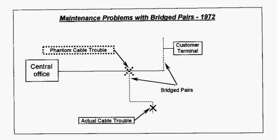
Whereas the previous diagram illustrates the maintenance reasons for eliminating bridged tap between a customer and the central office, the following diagram shows the existence of end section, which is electrically similar, but is bridged in parallel with the working line, going away from the customer's location, rather than between the customer and the central office.
