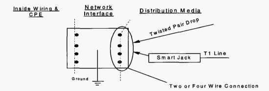
Figure 1 shows a schematic of a NID.
