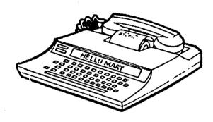
A TDD is a portable machine that looks like a typewriter. A user can send and receive typewritten messages to and from other TDDs via a telephone. For persons who also have visual impairments a large visual display or braille printer modification is available.
