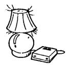
A Visual Ring Signaler connects to a light source (a lamp) and makes the light flash when the telephone rings.
