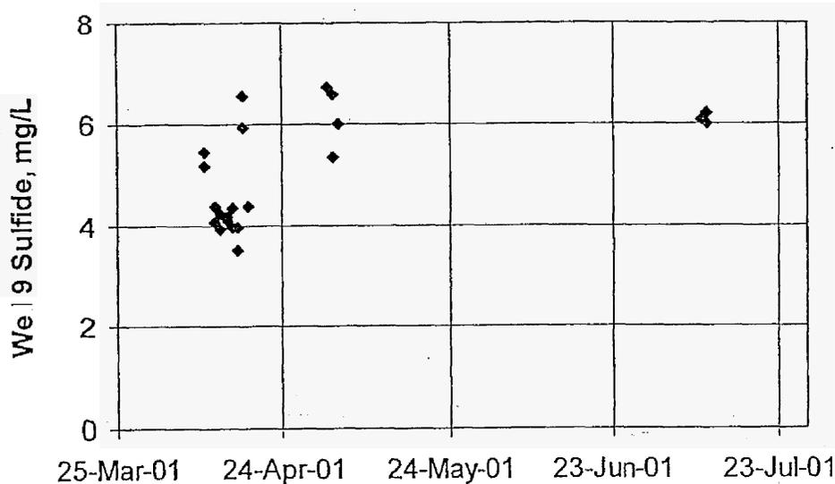
**Figure 10. Summary of hydrogen sulfide levels in untreated water from well 9 during a pilot study conducted to evaluate the effectiveness of ion exchange treatment (Data from Porter, 2002).**
