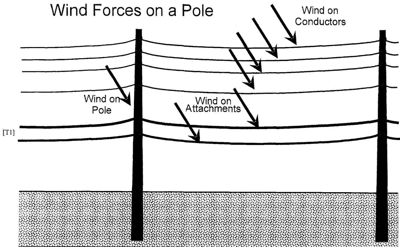
Wind loading creates a stress called “bending moment” on the pole. The force applied by the wind increases with the cross sectional area of items placed on the pole, not the weight.
