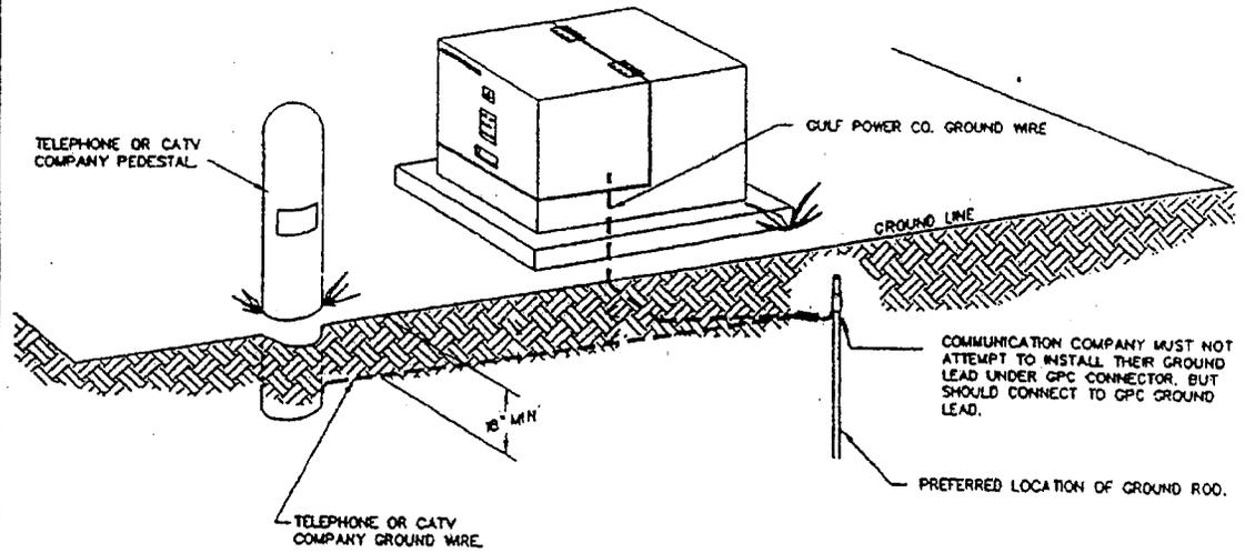
**ISOMETRIC VIEW OF TRANSFORMER PAD
