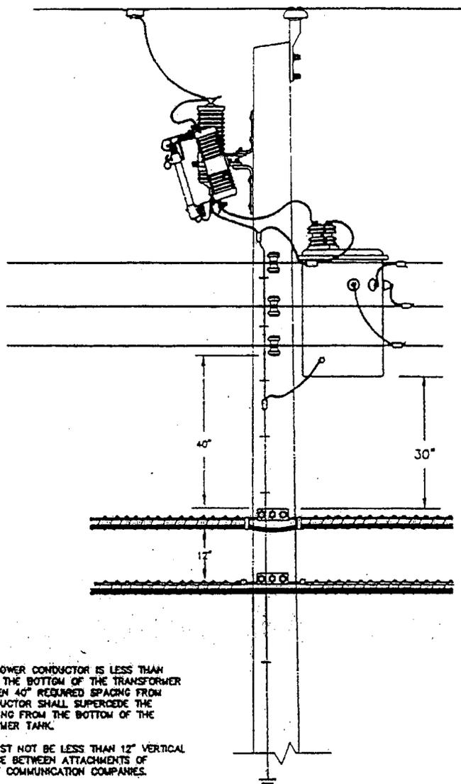
1. IF GULF POWER CONDUCTOR IS LESS THAN 10" FROM THE BOTTOM OF THE TRANSFORMER TANK, THEN 40" REQUIRED SPACING FROM THE CONDUCTOR SHALL SUPERCEDE THE 30" SPACING FROM THE BOTTOM OF THE TRANSFORMER TANK.
