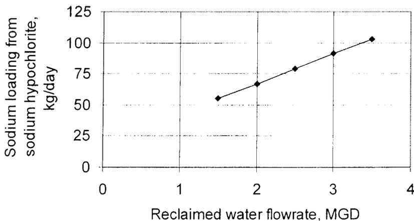
**Figure 16. Estimate of the amount of sodium discharged per day (kg/day) as a function of the reclaimed water flowrate at AUI's treatment facility.**
