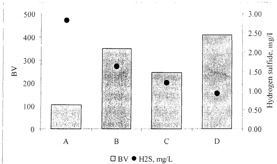
**Figure 6.** Comparison Between the Average Bed Volumes (volume of water/volume of resin) and the H<sub>2</sub>S Concentration at four treatment facilities: A: Plant 9, B: Plant 8, C: Plant 6, and D: Plant 2
