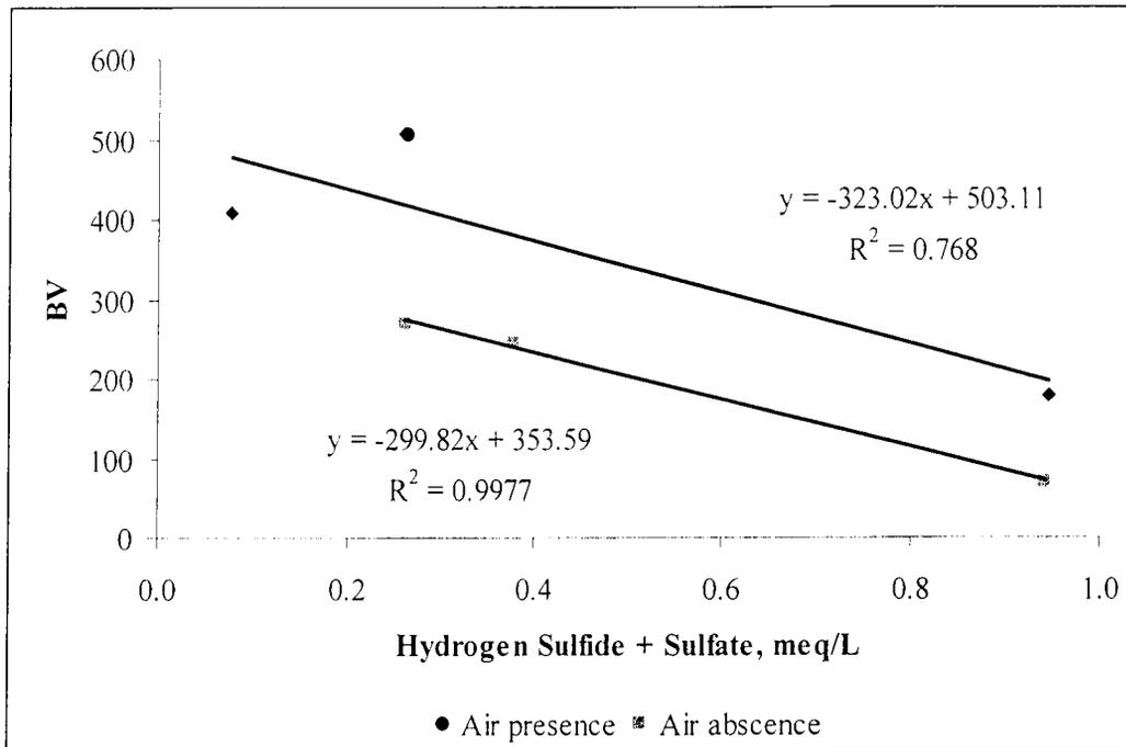
**Figure 11.** Relationship of the number of bed volumes for removal of hydrogen sulfide from Plants 2, 8, and 9 as a function of the concentration of exchangeable sulfur anions (sulfide and sulfate) in the presence or absence of upstream exposure to air.
