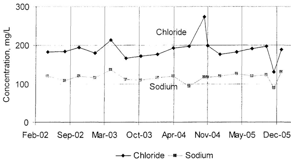
**Figure 14. Summary of chloride and sodium concentrations in AUI's reclaimed water from 2002 through 2005 (Data from Short Environmental Laboratories).**
