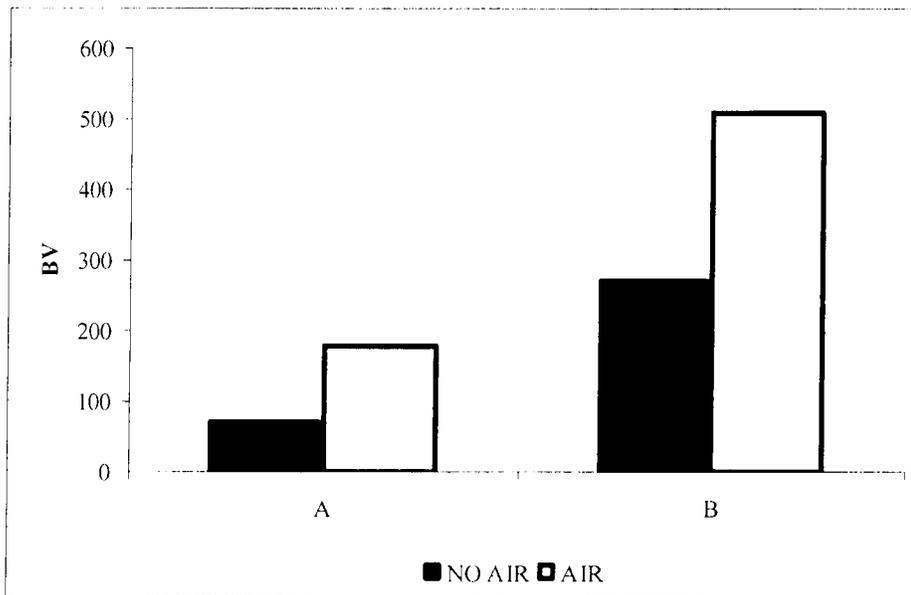
**Figure 10.** Comparison of the Average number of Bed Volumes for removal of hydrogen sulfide using Tulson® A-72 MP Resin in the presence or absence of Air at Plants 9 (A) and 8 (B).
