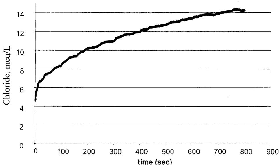
**Figure 5.** Example time series of chloride release during batch testing of anion exchange for uptake of hydrogen sulfide using Tulson® A-72 MP resin.
