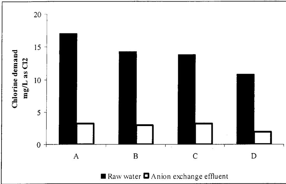
Figure 7. Comparison of Chlorine Demand in Water before and after Anion Exchange treatment at four treatment facilities: A: Plant 9, B: Plant 8, C: Plant 6, and D: Plant 2
