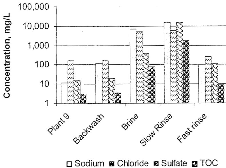
**Figure 1. Comparison of the concentrations of sodium, chloride, sulfate, and organic carbon (TOC) in waste streams from pilot-scale anion exchange testing at Plant 9 (note log-scale)**
