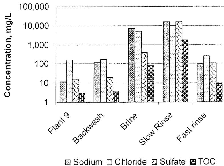
Figure 13. Comparison of the concentrations of sodium, chloride, sulfate, and organic carbon (TOC) in waste streams from pilot-scale anion exchange testing at Plant 9 (note log-scale)
