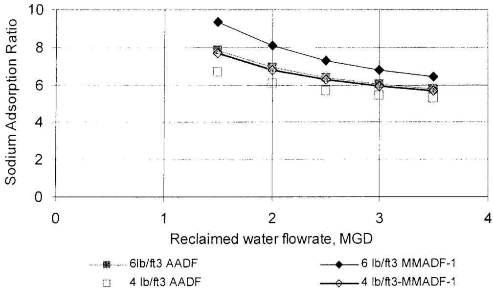
**Figure 18. Comparison of Sodium Adsorption Ratios (SAR) projected in reclaimed water that receives wastewater from anion exchange regeneration under two flow conditions: Average Annual Daily Flow (AADF) 2.04 MGD and Maximum Month Daily Flow (MMADF-1) 2.9 MGD. The wastewater flowrate is assumed to be 1.5 MGD.**
