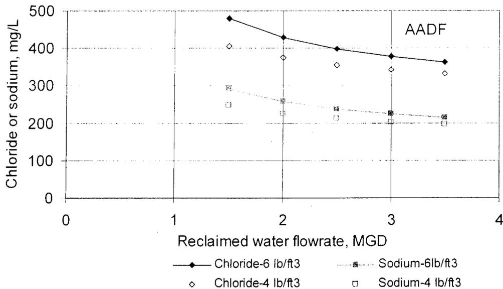
Figure 17. Estimated concentrations of chloride and sodium in reclaimed water under AADF operation of anion exchange reactors using either 4 or 6 lb of salt per cubic foot of resin.
