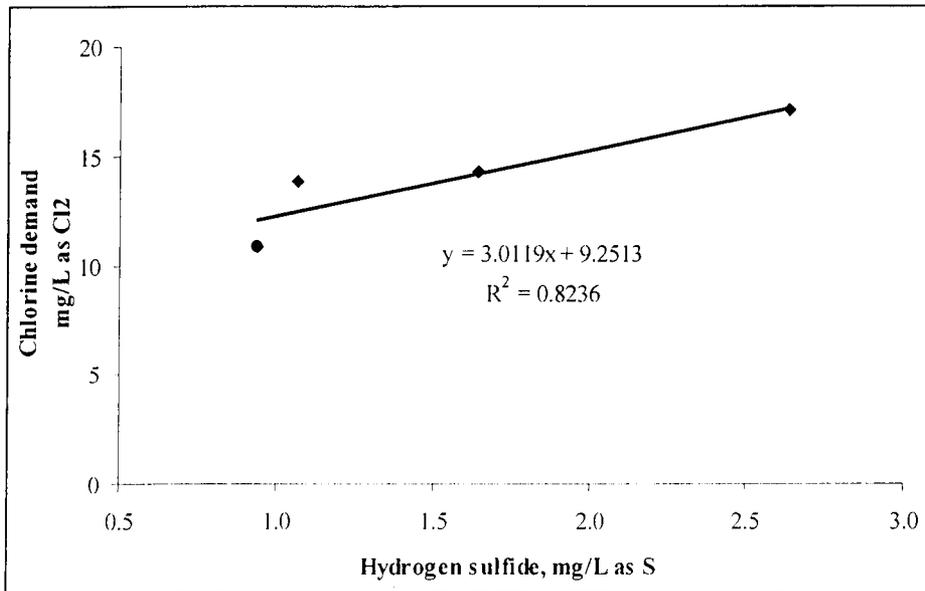
Figure 8. Chlorine Demand as Function of the Hydrogen Sulfide Concentration in untreated water from the Seven Spring service area.
