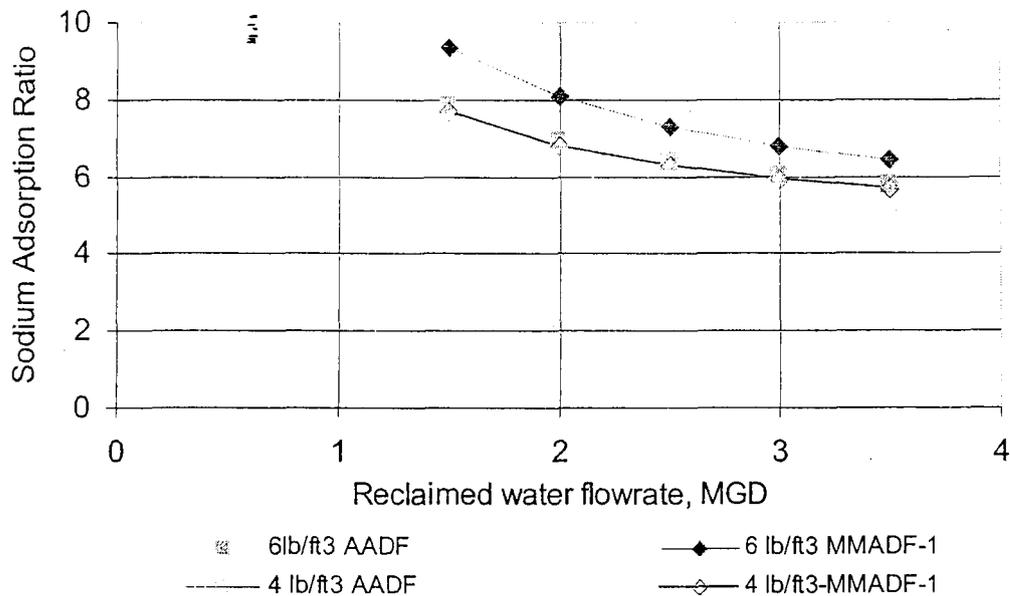
**Figure 6. Comparison of Sodium Adsorption Ratios (SAR) projected in reclaimed water that receives wastewater from anion exchange regeneration under two flow conditions: Average Annual Daily Flow (AADF) 2.04 MGD and Maximum Month Daily Flow (MMDF-1) 2.9 MGD. The wastewater flowrate is assumed to be 1.5 MGD.**
