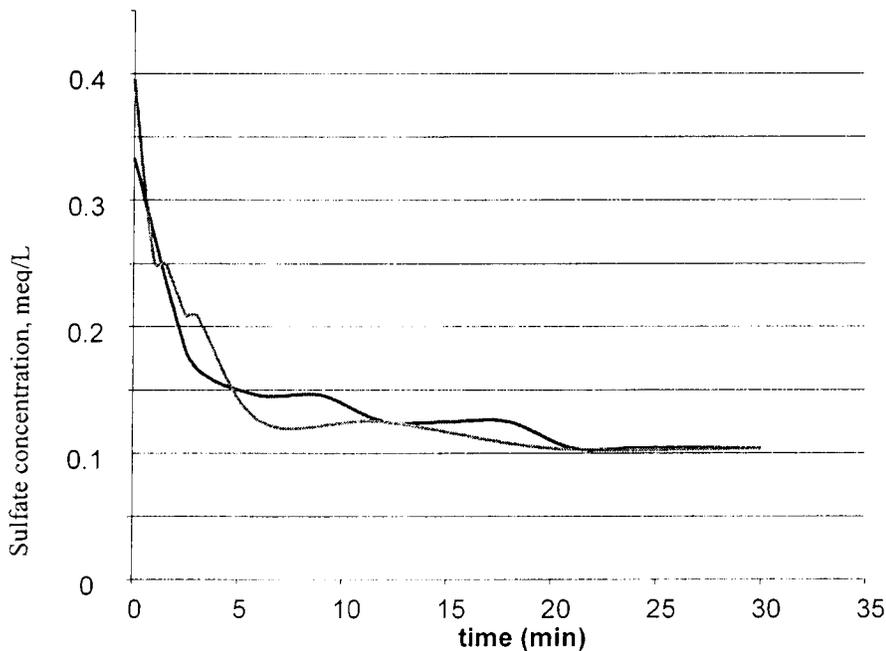
**Figure 4.** Anion exchange uptake of sulfate in batch tests conducted using Tulson® A-72 MP resin. The two lines represent two different batch tests.
