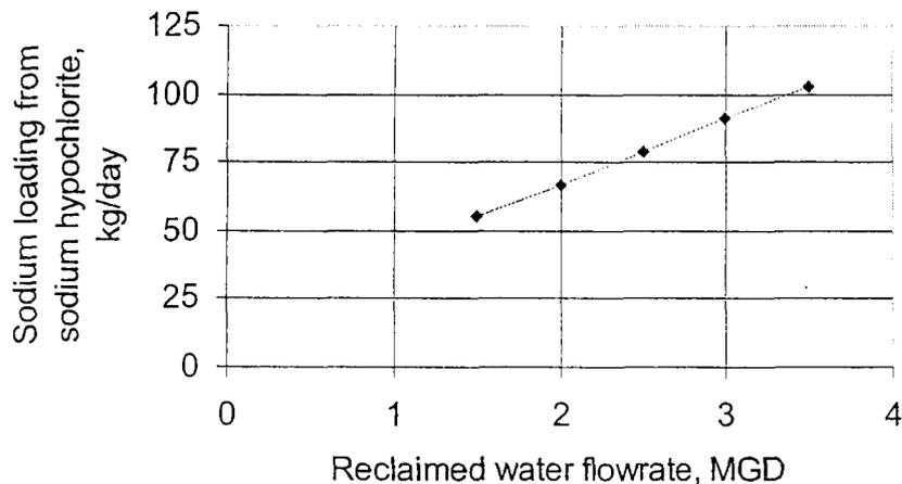
**Figure 4. Estimate of the amount of sodium discharged per day (kg/day) as a function of the reclaimed water flowrate at AUI's treatment facility.**
