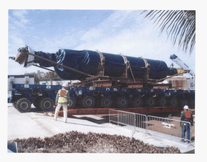
Unloading the Main Generator Rotor at St. Lucie Exhibit TOJ-17, Page 1 of 1
