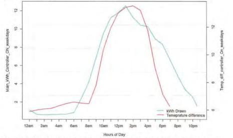
Figure 26: The figure above illustrates the relationship between the main disconnect kWh draw and the indoor and outdoor temperature difference when the controller is ON for the weekday hours (Monday to Friday). As it can be seen, as the temperature difference between indoor and outdoor temperature raises so does the kW consumption of the main disconnect panel. This indicates a high correlation between kW and temperature.
