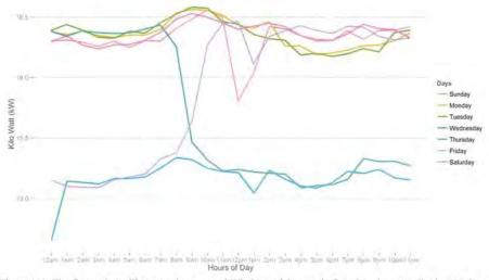
Figure 113: The figure above illustrates the average kWh draw of the supply fan when the controller is OFF for each hour of the day and each day of the week. This is helpful in understanding the operation of the unit throughout the days of the week. It is clear that as the temperature increases throughout the day, so will the kWh draw.
