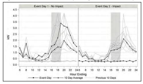
Figure 1-10: Illustration of Load Variability in a Single Home for Two Event Days
