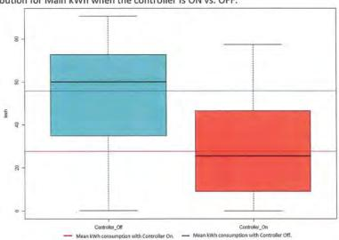
OFF) of 49.21% while maintaining the effect of the outside temperature. Figure displays the box plot distribution for Main kWh when the controller is ON vs. OFF.
