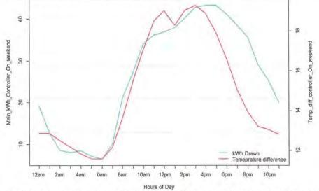
Figure 48: The figure above illustrates the relationship between the main disconnect kWh draw and the indoor and outdoor temperature difference when the controller is ON for the weekend hours (Saturday and Sunday). As it can be seen, as the temperature difference between indoor and outdoor temperature raises so does the kW consumption of the main disconnect panel. This indicates a high correlation between kW and temperature.
