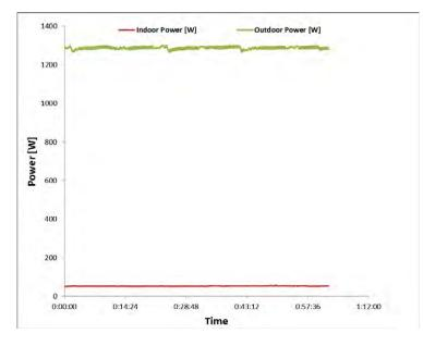
Figure 17: Solar test AHU and Condensing Unit electric power consumption (CASE II)
