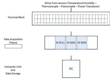
**Figure 4: Data Acquisition System**
