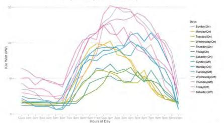
Figure 88: The figure above illustrates the average kWh draw of the compressors when the controller is ON and OFF for each hour of the day and each day of the week. This is helpful in understanding the operation of the unit throughout the days of the week. It is clear that as the temperature increases throughout the day, so will the kWh draw.
