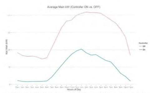
Figure 87: The plot above illustrates that there is a significant reduction in main kWh draw when the controller is ON versus when it is OFF. The kWh draw follows a similar trend throughout the day. This indicates that both control strategies are reacting to the outside temperature and super market occupancy.
