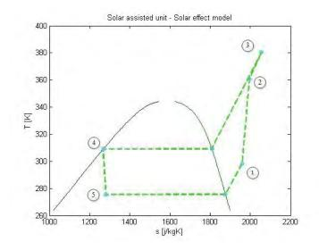
Figure 23: VCC T-s diagram - (CASE II)
