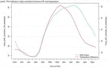
Figure 121: The figure above illustrates the relationship between the main disconnect kWh draw and the indoor and outdoor temperature difference when the controller is ON for the weekday hours (Monday to Friday). As it can be seen, as the temperature difference between indoor and outdoor temperature raises so does the kW consumption of the main disconnect panel. This indicates a high correlation between kW and temperature.
