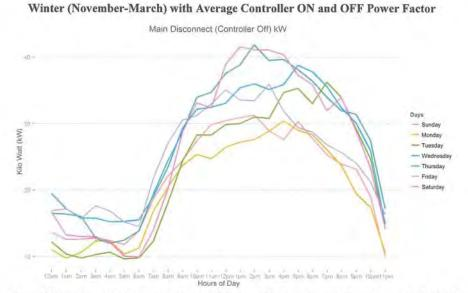
Figure 13: The figure above illustrates the average kWh draw of the main A/C unit when the controller is OFF for each hour of the day and each day of the week. This is helpful in understanding the operation of the unit throughout the days of the week. It is clear that as the temperature increases throughout the day, so will the kWh draw.
