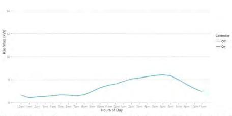
Figure 117: Figure above illustrates that there is a significant reduction in supply fan kWh draw when the controller is ON versus when it is OFF. The kWh draw follows a similar trend throughout the day. This indicates that both control strategies are reacting to the outside temperature and super market occupancy.
