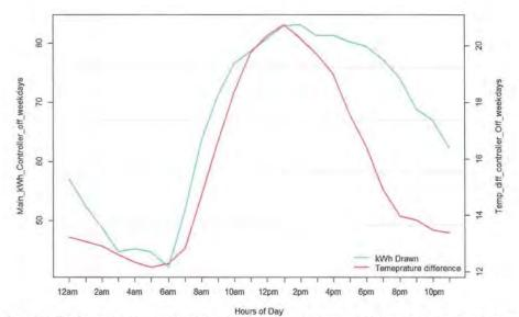
Figure 120: The figure above illustrates the relationship between the main disconnect kWh draw and the indoor and outdoor temperature difference when the controller is OFF for the weekday hours (Monday to Friday). As it can be seen, as the temperature difference between indoor and outdoor temperature increased so does the kW consumption of the main disconnect
