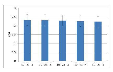
Figure 20: Solar test performance of the AC unit (CASE II)
