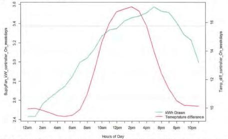
Figure 78: The figure above illustrates the relationship between the supply fan kWh draw and the indoor and outdoor temperature difference when the controller is ON for the weekday hours (Monday to Friday). As it can be seen, as the temperature difference between indoor and outdoor temperature raises so does the kW consumption of the main disconnect panel. This indicates a high correlation between kW and temperature.
