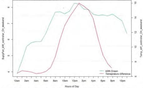
Figure 99: The figure above illustrates the relationship between the supply fan kWh draw and the indoor and outdoor temperature difference when the controller is ON for the weekend hours (Saturday and Sunday). As it can be seen, as the temperature difference between indoor and outdoor temperature raises so does the kW consumption of the main disconnect panel. This indicates a high correlation between kW and temperature.
