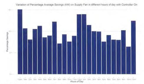
Figure 140: The figure above illustrates the average percent savings of the supply fan throughout the day. As it can be seen, savings are higher during the cooler parts of the day as the VFD is able to slow down he speed of the fan for longer periods of time.
