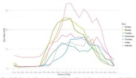
Figure 86: The figure above illustrates the average kWh draw of the main disconnect when the controller is ON for each hour of the day and each day of the week. This is helpful in understanding the operation of the unit throughout the days of the week. It is clear that as the temperature increases throughout the day, so will the kWh draw.
