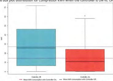
controller is OFF) of 45.54% while maintaining the effect of the outside temperature. Figure displays the box plot distribution for Compressor kWh when the controller is ON vs. OFF.
