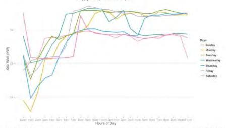
Figure 137: The figure above illustrates the average kWh draw of the supply fan when the controller is OFF for each hour of the day and each day of the week. This is helpful in understanding the operation of the unit throughout the days of the week. It is clear that as the temperature increases throughout the day, so will the kWh draw.
