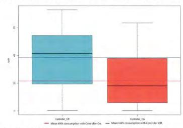
controller is OFF) of 42.30% while maintaining the effect of the outside temperature. Figure displays the box plot distribution for Compressor kWh when the controller is ON vs. OFF.
