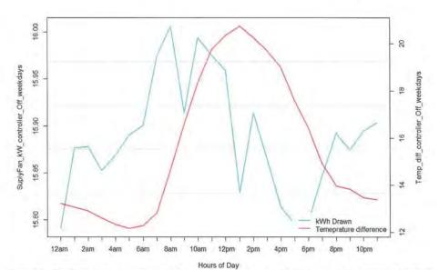
Figure 124: The figure above illustrates the relationship between the supply fan kWh draw and the indoor and outdoor temperature difference when the controller is OFF for the weekday hours (Monday to Friday). As it can be seen, as the temperature difference between indoor and outdoor temperature increased so does the kW consumption of the main disconnect panel. This indicates a high correlation between kW and temperature.
