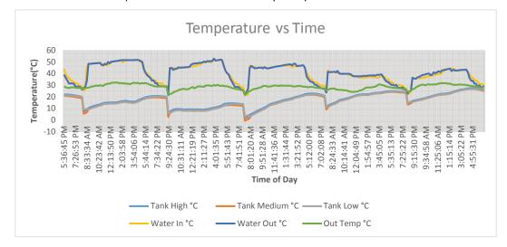
Total energy generation of both types of panels are calculated by using the aggregate data a sample of which is shown in Figure 3.1 and the results are summarized in Table 3.1. The cooled PVTs generate about 20% more energy on average more than the uncooled PVTs. It should be noted the reported values are based on measured real data affected by actual weather conditions such as overcast and rain. And therefore lower than the maximum efficiency reported in the spec sheets of the panels.
