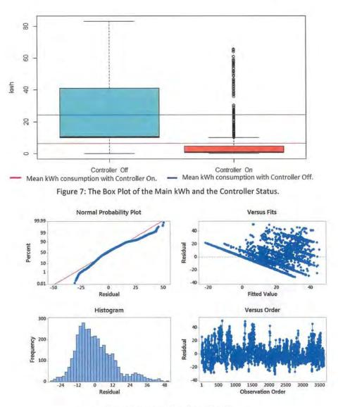
Figure 8: Residual Plots for Main kWh.
