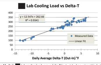
Figure 11. Daily Lab cooling load versus delta-T (out – in) when using attic ducts.
