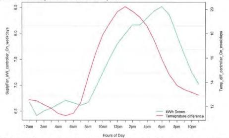
Figure 125: The figure above illustrates the relationship between the supply fan kWh draw and the indoor and outdoor temperature difference when the controller is ON for the weekday hours (Monday to Friday). As it can be seen, as the temperature difference between indoor and outdoor temperature raises so does the kW consumption of the main disconnect panel. This indicates a high correlation between kW and temperature.
