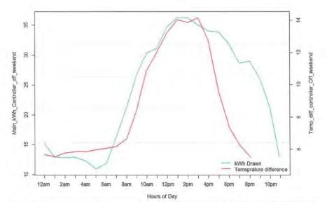
Figure 23: The figure above illustrates the relationship between the main disconnect kWh draw and the indoor and outdoor temperature difference when the controller is OFF for the weekend hours (Saturday and Sunday). As it can be seen, as the temperature difference between indoor and outdoor temperature increased so does the kW consumption of the main disconnect panel. This indicates a high correlation between kW and temperature.
