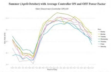
Figure 37: The figure above illustrates the average kWh draw of the main disconnect when the controller is OFF for each hour of the day and each day of the week. This is helpful in understanding the operation of the unit throughout the days of the week. It is clear that as the temperature increases throughout the day, so will the kWh draw.
