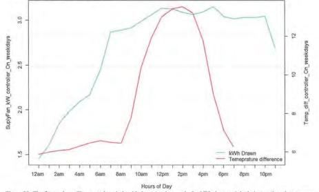
Figure 30: The figure above illustrates the relationship between the supply fan kWh draw and the indoor and outdoor temperature difference when the controller is ON for the weekday hours (Monday to Friday). As it can be seen, as the temperature difference between indoor and outdoor temperature raises so does the kW consumption of the main disconnect panel. This indicates a high correlation between kW and temperature.
