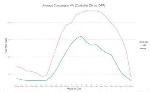
Figure 89: The plot above that there is a significant reduction in compressor kWh draw when the controller is ON versus when it is OFF. The kWh draw follows a similar trend throughout the day. This indicates that both control strategies are reacting to the outside temperature and super market occupancy.
