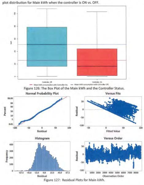
OFF) of 49.14% while maintaining the effect of the outside temperature. Figure displays the box plot distribution for Main kWb when the controller is ON vs. OFF
