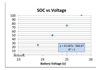
Figure 6. Battery SOC versus Battery Resting Voltage (data from battery manufacturer).
