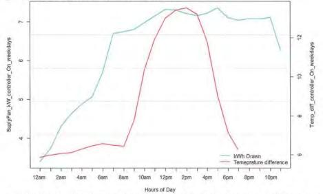
Figure 101: The figure above illustrates the relationship between the supply fan kWh draw and the indoor and outdoor temperature difference when the controller is ON for the weekday hours (Monday to Friday). As it can be seen, as the temperature difference between indoor and outdoor temperature raises so does the kW consumption of the main disconnect panel. This indicates a high correlation between kW and temperature.
