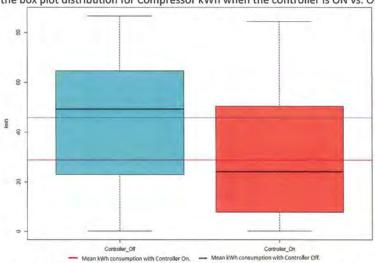
controller is OFF) of 35.49% while maintaining the effect of the outside temperature. Figure displays the box plot distribution for Compressor kWh when the controller is ON vs. OFF.
