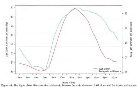
Figure 49: The figure above illustrates the relationship between the main disconnect kWh draw and the indoor and outdoor temperature difference when the controller is OFF for the weekday hours (Monday to Friday). As it can be seen, as the temperature difference between indoor and outdoor temperature increased so does the kW consumption of the main disconnect panel. This indicates a high correlation between kW and temperature.
