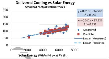
Figure 9. Cooling energy delivered by the solar heat pump system as a function of daily solar radiation for <u>Standard</u> thermostat control mode when using the eight battery storage bank.
