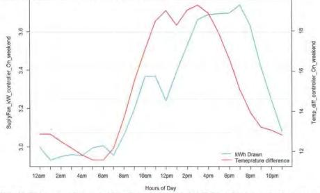
Figure 52: The figure above illustrates the relationship between the supply fan kWh draw and the indoor and outdoor temperature difference when the controller is ON for the weekend hours (Saturday and Sunday). As it can be seen, as the temperature difference between indoor and outdoor temperature raises so does the kW consumption of the main disconnect panel. This indicates a high correlation between kW and temperature.
