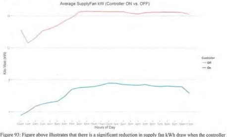
Figure 93: Figure above illustrates that there is a significant reduction in supply fan kWh draw when the controller is ON versus when it is OFF. The kWh draw follows a similar trend throughout the day. This indicates that both control strategies are reacting to the outside temperature and super market occupancy.
