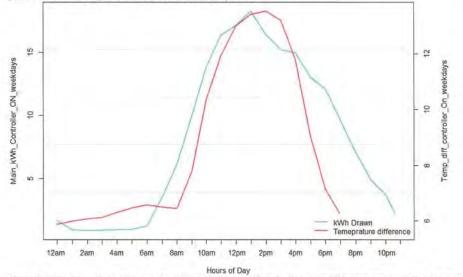
Figure 97: The figure above illustrates the relationship between the main disconnect kWh draw and the indoor and outdoor temperature difference when the controller is ON for the weekday hours (Monday to Friday). As it can be seen, as the temperature difference between indoor and outdoor temperature raises so does the kW consumption of the main disconnect panel. This indicates a high correlation between kW and temperature.
