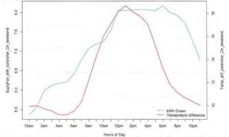
Figure 147: The figure above illustrates the relationship between the supply fan kWh draw and the indoor and outdoor temperature difference when the controller is ON for the weekend hours (Saturday and Sunday). As it can be seen, as the temperature difference between indoor and outdoor temperature raises so does the kW consumption of the main disconnect panel. This indicates a high correlation between kW and temperature.
