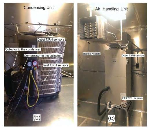
Figure 6: (a) solar collector, (b) condensing unit and (c) air handling unit
