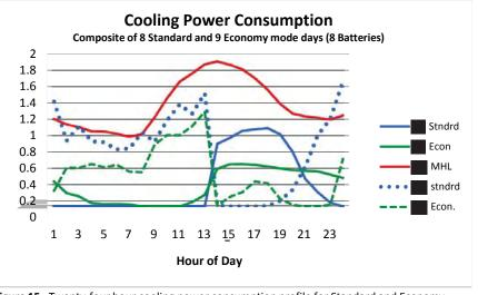
Figure 15. Twenty-four hour cooling power consumption profile for Standard and Economy mini-split operation when using 8 batteries, plus cooling power consumption for the Lab SEER 13 central system. Figure 15 has added economy profile to Figure 14.
