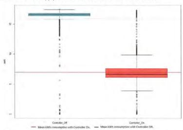
OFF) of 56.0% while maintaining the effect of the outside temperature. Figure 7 displays the box plot distribution for Supply Fan kWh when the controller is ON vs. OFF.
