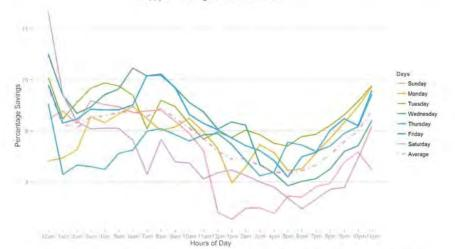
Figure 139: From the above plot we can infer comparing with a referential point; here we consider the average savings, how the savings in a specific day of the week and a specific hour of the day varies from the savings reference. We can see from the plot that variation of average hourly kilowatt savings on Sunday (Orange) and Saturday (Purple) are lesser to the average savings comparing with the two extreme weekdays i.e. Tuesday (Sea
