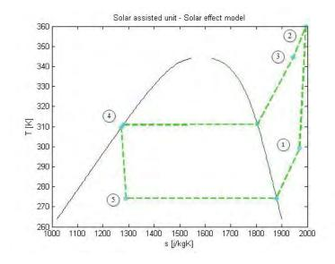
Figure 24: VCC T-s diagram - (CASE I)
