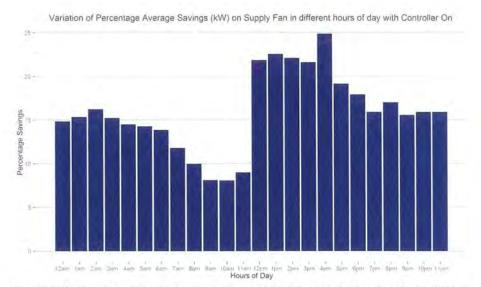
Figure 116: The figure above illustrates the average percent savings of the supply fan throughout the day. As it can be seen, savings are higher during the cooler parts of the day as the VFD is able to slow down he speed of the fan for longer periods of time.
