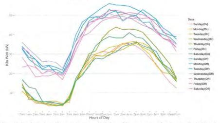
Figure 40: The figure above illustrates the average kWh draw of the compressors when the controller is ON and OFF for each hour of the day and each day of the week. This is helpful in understanding the operation of the unit throughout the days of the week. It is clear that as the temperature increases throughout the day, so will the kWh draw.
