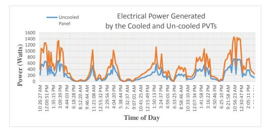
**Figure 3-1:** Electrical power generated by the cooled and un-cooled PVTs for a period of 5 days in 9/21/2014 - 9/26/2014.
