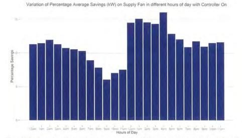
Figure 45: The figure above illustrates the average percent savings of the supply fan throughout the day. As it can be seen, savings are higher during the cooler parts of the day as the VFD is able to slow down he speed of the fan for longer periods of time.
