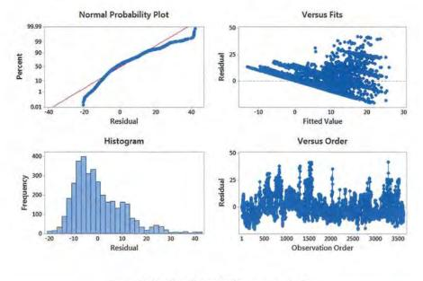
Figure 10: Residual Plots for Compressor kWh
