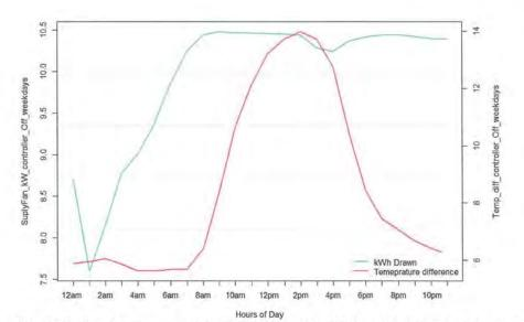
Figure 29: The figure above illustrates the relationship between the supply fan kWh draw and the indoor and outdoor temperature difference when the controller is OFF for the weekday hours (Monday to Friday). As it can be seen, as the temperature difference between indoor and outdoor temperature increased so does the kW consumption of the main disconnect panel. This indicates a high correlation between kW and temperature.
