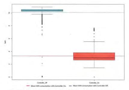
Figure 35: The Box Plot of the Supply Fan kWh and the Controller Status.
