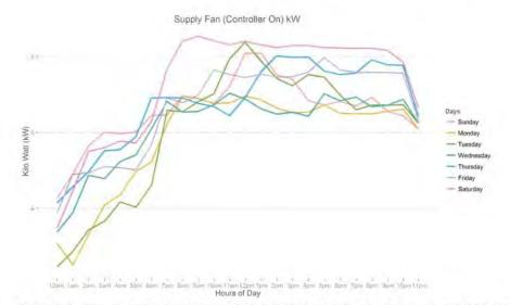
Figure 91: The figure above illustrates the average kWh draw of the supply fan when the controller is ON for each hour of the day and each day of the week. This is helpful in understanding the operation of the unit throughout the days of the week. It is clear that as the temperature increases throughout the day, so will the kWh draw.
