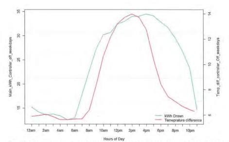
Figure 25: The figure above illustrates the relationship between the main disconnect kWh draw and the indoor and outdoor temperature difference when the controller is OFF for the weekday hours (Monday to Friday). As it can be seen, as the temperature difference between indoor and outdoor temperature increased so does the kW consumption of the main disconnect panel. This indicates a high correlation between kW and temperature.
