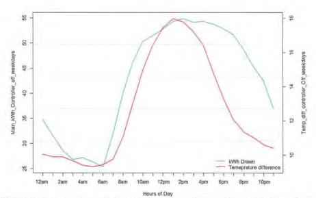
Figure 73: The figure above illustrates the relationship between the main disconnect kWh draw and the indoor and outdoor temperature difference when the controller is OFF for the weekday hours (Monday to Friday). As it can be seen, as the temperature difference between indoor and outdoor temperature increased so does the kW consumption of the main disconnect panel. This indicates a high correlation between kW and temperature.
