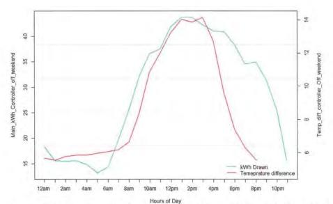
Figure 94: The figure above illustrates the relationship between the main disconnect kWh draw and the indoor and outdoor temperature difference when the controller is OFF for the weekend hours (Saturday and Sunday). As it can be seen, as the temperature difference between indoor and outdoor temperature increased so does the kW consumption of the main disconnect panel. This indicates a high correlation between kW and temperature.
