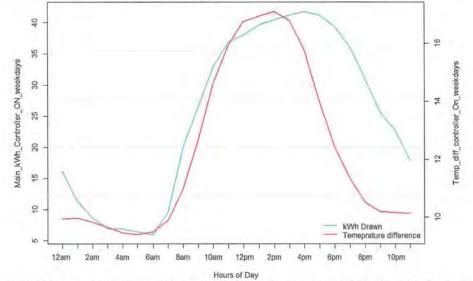
Figure 145: The figure above illustrates the relationship between the main disconnect kWh draw and the indoor and outdoor temperature difference when the controller is ON for the weekday hours (Monday to Friday). As it can be seen, as the temperature difference between indoor and outdoor temperature raises so does the kW consumption of the main disconnect panel. This indicates a high correlation between kW and temperature.
