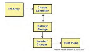
Figure 25. "As-tested" Stand-Alone Solar Heat Pump System
