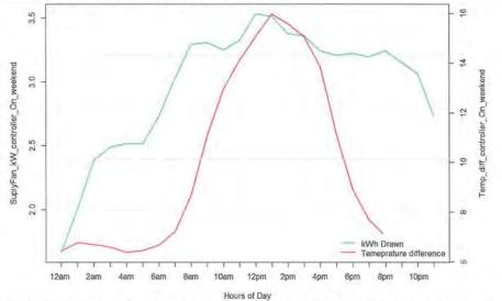
Figure 28: The figure above illustrates the relationship between the supply fan kWh draw and the indoor and outdoor temperature difference when the controller is ON for the weekend hours (Saturday and Sunday). As it can be seen, as the temperature difference between indoor and outdoor temperature raises so does the kW consumption of the main disconnect panel. This indicates a high correlation between kW and temperature.
