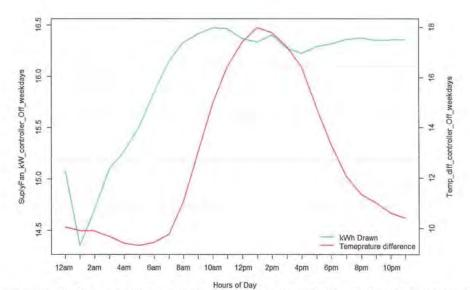
Figure 148: The figure above illustrates the relationship between the supply fan kWh draw and the indoor and outdoor temperature difference when the controller is OFF for the weekday hours (Monday to Friday). As it can be seen, as the temperature difference between indoor and outdoor temperature increased so does the kW consumption of the main disconnect panel. This indicates a high correlation between kW and temperature.
