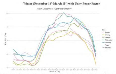
Figure 85: The figure above illustrates the average kWh draw of the main disconnect when the controller is OFF for each hour of the day and each day of the week. This is helpful in understanding the operation of the unit throughout the days of the week. It is clear that as the temperature increases throughout the day, so will the kWh draw.
