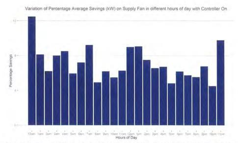
Figure 69: The figure above illustrates the average percent savings of the supply fan throughout the day. As it can be seen, savings are higher during the cooler parts of the day as the VFD is able to slow down he speed of the fan for longer periods of time.
