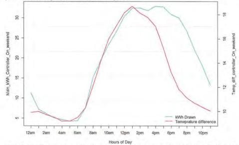
Figure 72: The figure above illustrates the relationship between the main disconnect kWh draw and the indoor and outdoor temperature difference when the controller is ON for the weekend hours (Saturday and Sunday). As it can be seen, as the temperature difference between indoor and outdoor temperature raises so does the kW consumption of the main disconnect panel. This indicates a high correlation between kW and temperature.
