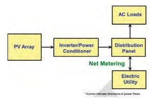
Figure 23. Utility Grid-Interactive PV System
