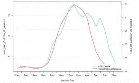
Figure 24: The figure above illustrates the relationship between the main disconnect kWh draw and the indoor and outdoor temperature difference when the controller is ON for the weekend hours (Saturday and Sunday). As it can be seen, as the temperature difference between indoor and outdoor temperature raises so does the kW consumption of the main disconnect panel. This indicates a high correlation between kW and temperature.
