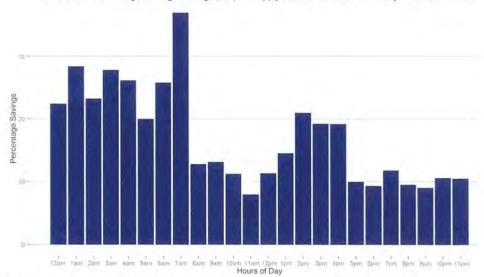
Variation of Percentage Average Savings (kW) on Supply Fan in different hours of day with Controller On
