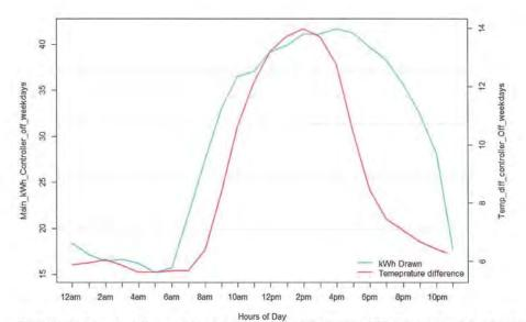
Figure 96: The figure above illustrates the relationship between the main disconnect kWh draw and the indoor and outdoor temperature difference when the controller is OFF for the weekday hours (Monday to Friday). As it can be seen, as the temperature difference between indoor and outdoor temperature increased so does the kW consumption of the main disconnect panel. This indicates a high correlation between kW and temperature.
