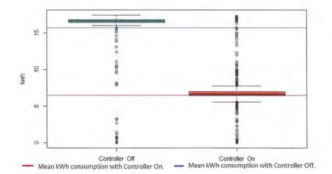
Figure 83: The Box Plot of the Supply Fan kWh and the Controller Status.
