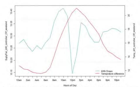
Figure 51: The figure above illustrates the relationship between the supply fan kWh draw and the indoor and outdoor temperature difference when the controller is OFF for the weekend hours (Saturday and Sunday). As it can be seen, as the temperature difference between indoor and outdoor temperature increased so does the kW consumption of the main disconnect panel. This indicates a high correlation between kW and temperature.
