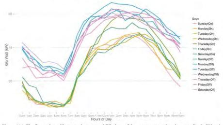
Figure 111: The figure above illustrates the average kWh draw of the compressors when the controller is ON and OFF for each hour of the day and each day of the week. This is helpful in understanding the operation of the unit throughout the days of the week. It is clear that as the temperature increases throughout the day, so will the kWh draw.
