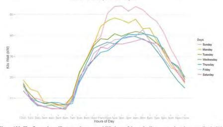
Figure 133: The figure above illustrates the average kWh draw of the main disconnect when the controller is ON for each hour of the day and each day of the week. This is helpful in understanding the operation of the unit throughout the days of the week. It is clear that as the temperature increases throughout the day, so will the kWh draw.
