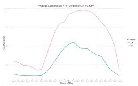
Figure 17: The figure above illustrates that there is a significant reduction in compressor kWh draw when the controller is ON versus when it is OFF. The kWh draw follows a similar trend throughout the day. This indicates that both control strategies are reacting to the outside temperature and super market occupancy.
