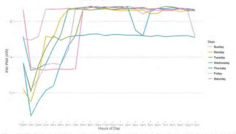
Figure 90: The figure above illustrates the average kWh draw of the supply fan when the controller is OFF for each hour of the day and each day of the week. This is helpful in understanding the operation of the unit throughout the days of the week. It is clear that as the temperature increases throughout the day, so will the kWh draw.
