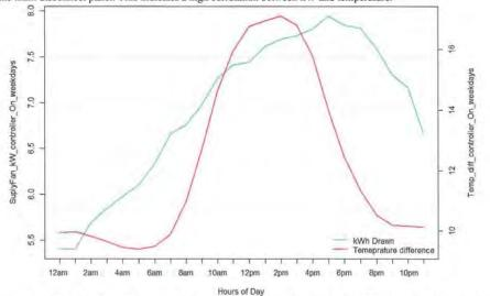
Figure 149: The figure above illustrates the relationship between the supply fan kWh draw and the indoor and outdoor temperature difference when the controller is ON for the weekday hours (Monday to Friday). As it can be seen, as the temperature difference between indoor and outdoor temperature raises so does the kW consumption of the main disconnect panel. This indicates a high correlation between kW and temperature.
