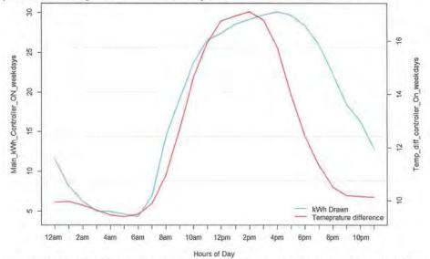
Figure 74: The figure above illustrates the relationship between the main disconnect kWh draw and the indoor and outdoor temperature difference when the controller is ON for the weekday hours (Monday to Friday). As it can be seen, as the temperature difference between indoor and outdoor temperature raises so does the kW consumption of the main disconnect panel. This indicates a high correlation between kW and temperature.
