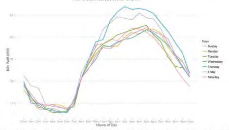
Figure 38: The figure above illustrates the average kWh draw of the main disconnect when the controller is ON for each hour of the day and each day of the week. This is helpful in understanding the operation of the unit throughout the days of the week. It is clear that as the temperature increases throughout the day, so will the kWh draw.
