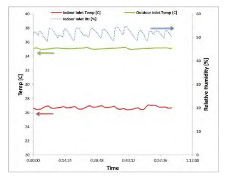
Figure 16: Solar test conditions for rooms A and B (CASE II)
