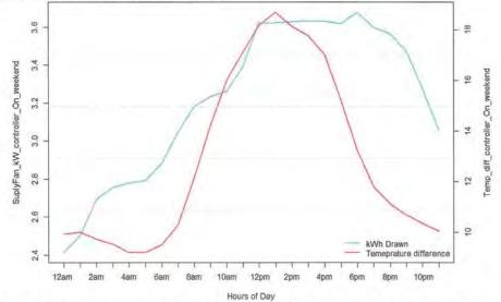
Figure 76: The figure above illustrates the relationship between the supply fan kWh draw and the indoor and outdoor temperature difference when the controller is ON for the weekend hours (Saturday and Sunday). As it can be seen, as the temperature difference between indoor and outdoor temperature raises so does the kW consumption of the main disconnect panel. This indicates a high correlation between kW and temperature.
