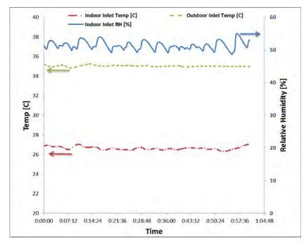
Figure 8: Bypass test conditions for rooms A and B
