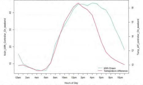
Figure 143: The figure above illustrates the relationship between the main disconnect kWh draw and the indoor and outdoor temperature difference when the controller is ON for the weekend hours (Saturday and Sunday). As it can be seen, as the temperature difference between indoor and outdoor temperature raises so does the kW consumption of the main disconnect panel. This indicates a high correlation between kW and temperature.
