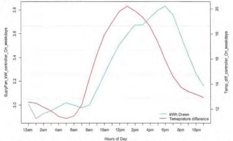
Figure 54: The figure above illustrates the relationship between the supply fan kWh draw and the indoor and outdoor temperature difference when the controller is ON for the weekday hours (Monday to Friday). As it can be seen, as the temperature difference between indoor and outdoor temperature raises so does the kW consumption of the main disconnect panel. This indicates a high correlation between kW and temperature.
