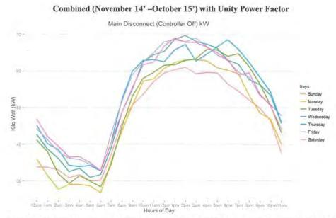
Figure 132: The figure above illustrates the average kWh draw of the main disconnect when the controller is OFF for each hour of the day and each day of the week. This is helpful in understanding the operation of the unit throughout the days of the week. It is clear that as the temperature increases throughout the day, so will the kWh draw.
