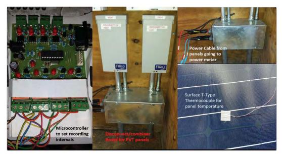
Figure 2-7 Microcontroller, DC-disconnect/Combiner, Surface thermocouple.
