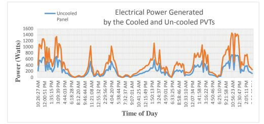
**Figure 1.1:** Electrical power generated by the cooled and un-cooled PVTs for a period of 5 days in 9/21/2014 - 9/26/2014.
