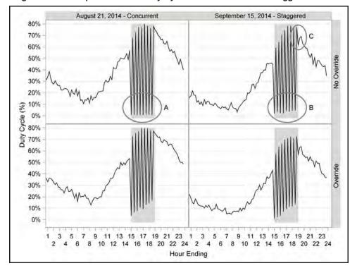
Figure 1-13: Comparison of AC Duty Cycles for Concurrent vs. Staggered Rollout
