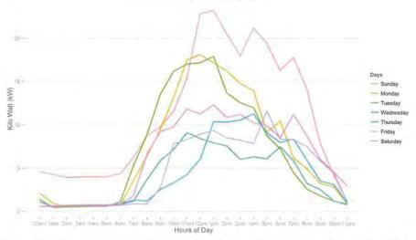
Figure 14: The figure above illustrates the average kWh draw of the main A/C unit when the controller is ON for each hour of the day and each day of the week. This is helpful in understanding the operation of the unit throughout the days of the week. It is clear that as the temperature increases throughout the day, so will the kWh draw.
