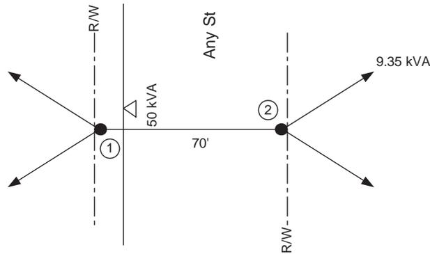
From Table III, 4 full electric customers with 3 1/2 ton A/C require a 50 kVA transformer.
