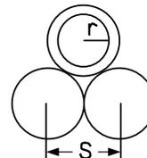
In section ii and iii, reactance values were calculated using the above formula with conductor diameter and insulation thickness per FPL specifications.
