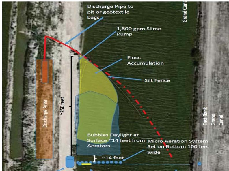
Figure C-1 Arrangement of Direct Treatment Pilot Study Equipment
