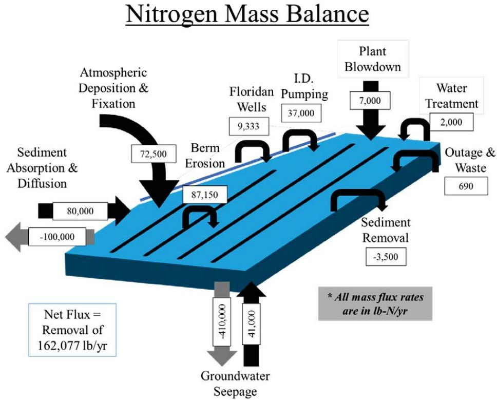
Figure A.1 – Nitrogen Mass Balance for Turkey Point CCS using data of Table 2.3
