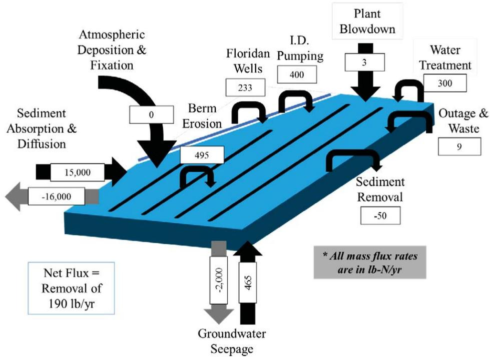
Figure A.2 - Phosphorous Mass Balance for Turkey Point CCS using data of Table 2.3
