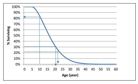
Figure 2: Example Survival Function for ENERGY STAR® Refrigerators
