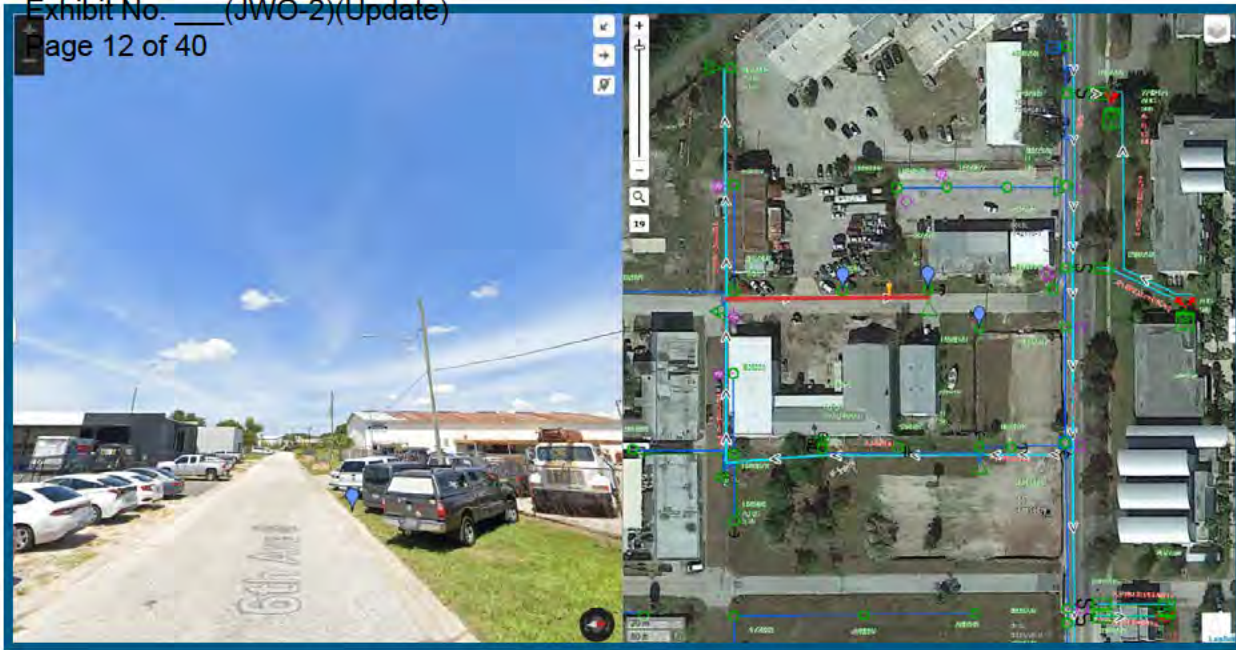
Figure 3: The teal tap line branches off the main road through an open lot to side streets where it splits again. It serves a few customers with minimal, to no vegetation. The street view is a view of the red line where there are no vegetation concerns.
