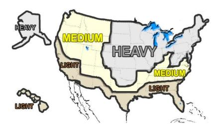
Figure 2: NESC General loading map of United States with respect to loading of overhead lines.
