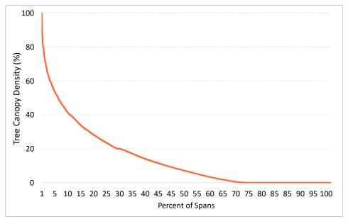
Figure 4-3: Vegetation Density on TEC Transmission Conductor
