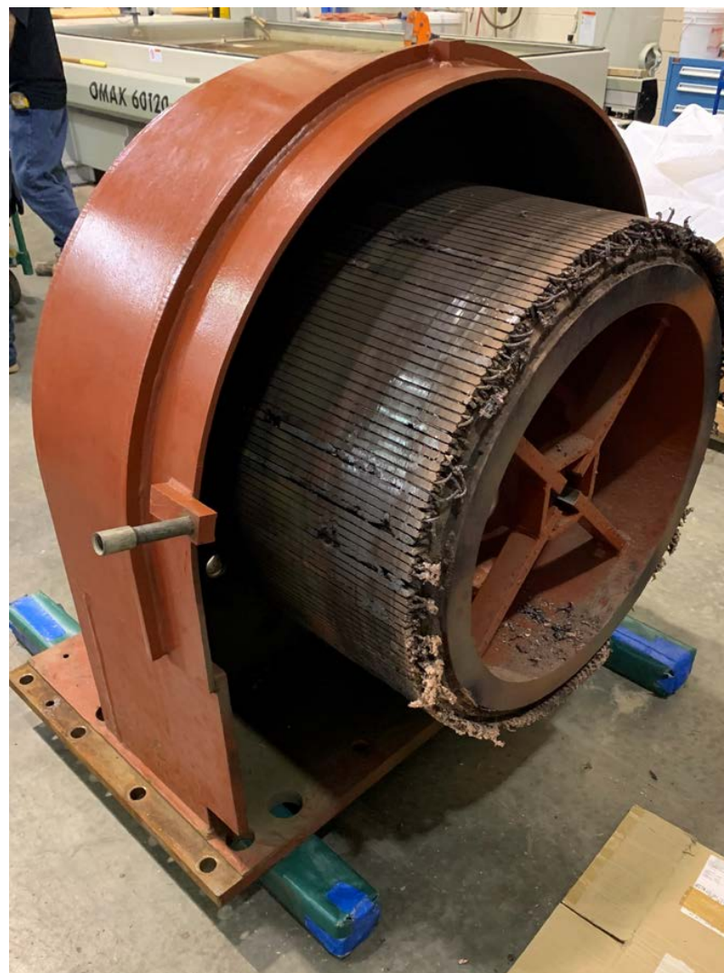
Fig. 5 U4 PMG Stator Removed
