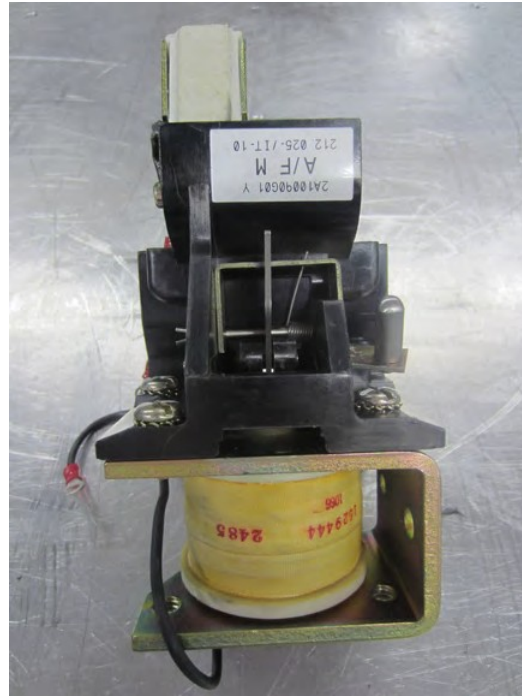
Rear of Control Relay
