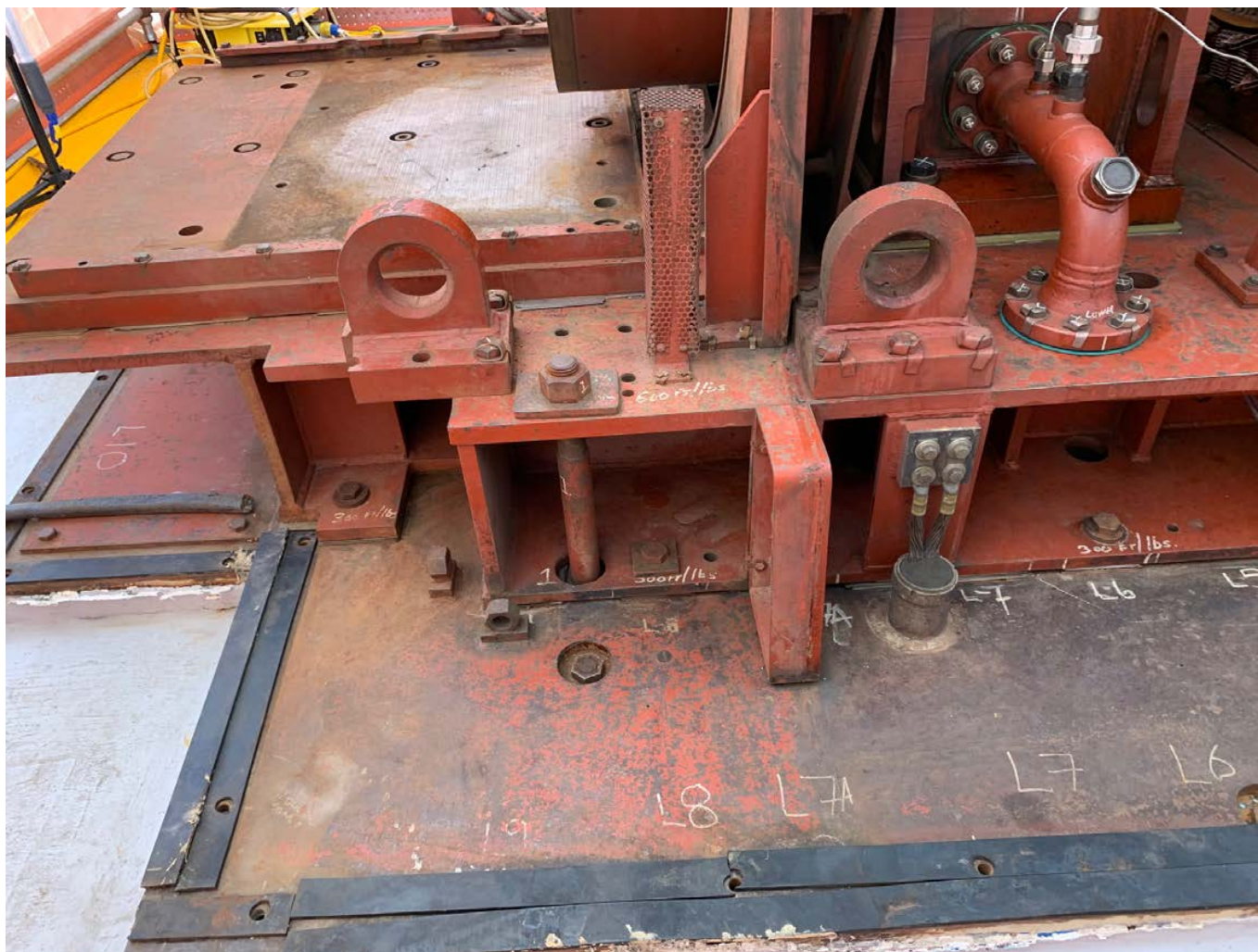
Fig. 13 Exciter Base to Housing Seal / Gasket Arrangement
