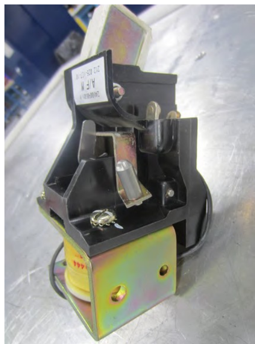
Other Side of Control Relay
