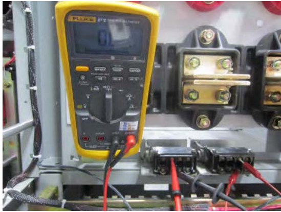
Right-Side Switch Monitoring (NO)
