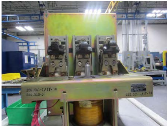
Breaker with the Operating Mechanism Removed
