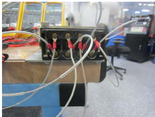
Right-Side Switch Monitoring Connections
