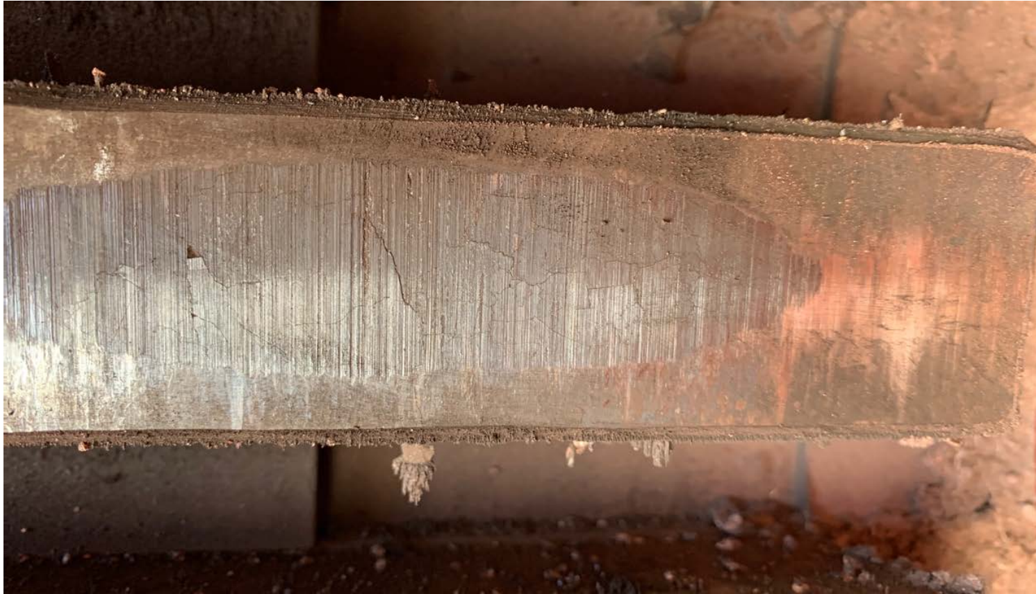
Fig. 10 PMG Magnet Cracking
