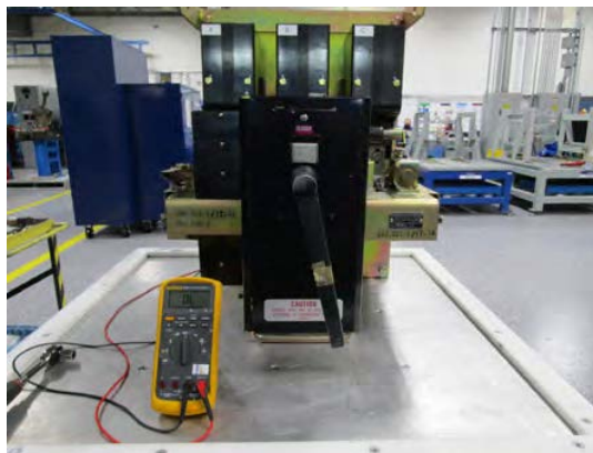
Breaker Closed, Switch Contact Open
