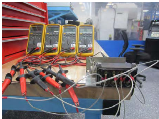
Right-Side Switch Monitoring
