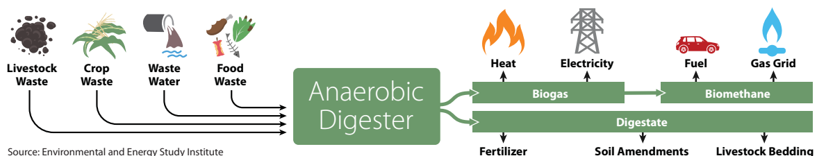
Figure 1: Anaerobic Digestion Process
