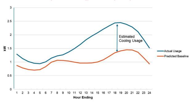
Figure 9: Methodology for Estimating Cooling Loads
