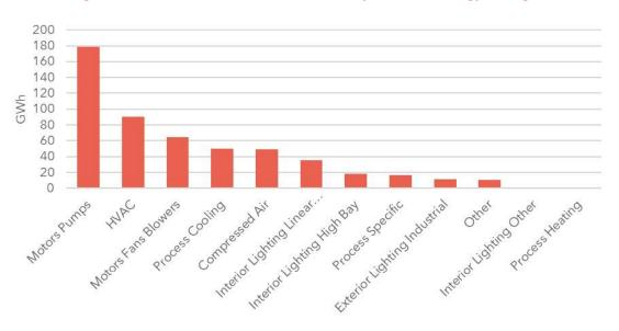
Figure 19: Industrial EE Technical Potential by End-Use (Energy Savings)
