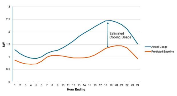
Figure 9: Methodology for Estimating Cooling Loads
