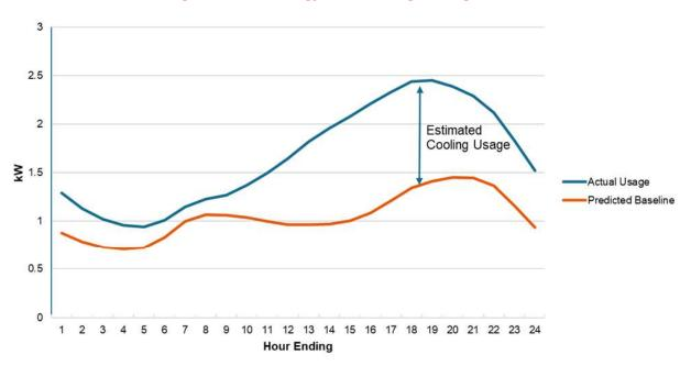
Figure 7: Methodology for Estimating Cooling Loads
