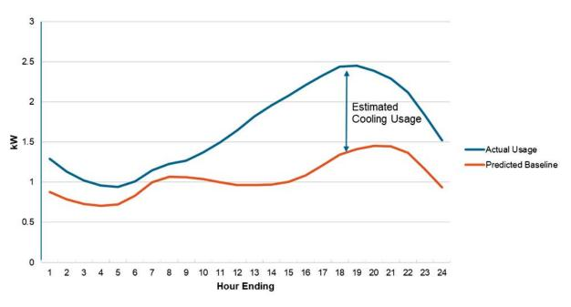
Figure 9: Methodology for Estimating Cooling Loads
