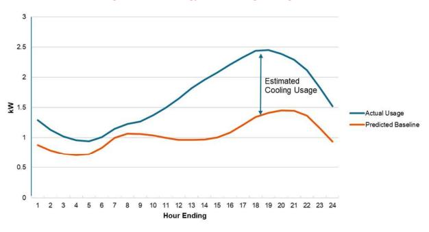
Figure 9: Methodology for Estimating Cooling Loads
