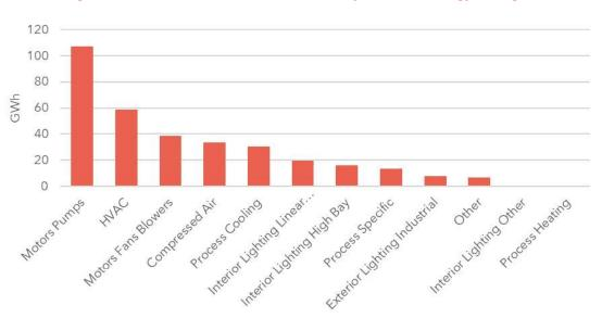
Figure 19: Industrial EE Technical Potential by End-Use (Energy Savings)
