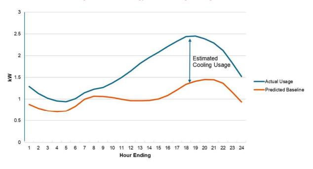
Figure 9: Methodology for Estimating Cooling Loads
