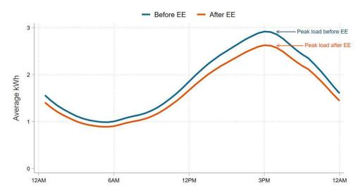
Figure 10: Illustration of EE Impacts on HVAC System Load Shape
