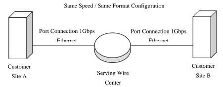
This example illustrates a 1Gbps Ethernet circuit from Customer Site A to Customer Site B for a same speed / same format arrangement. In this example, two – 1Gbps Ethernet Port Connection charges are applicable.
