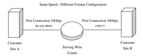
This example illustrates a same speed / different format circuit configuration whereby there is a 10Gbps WAN-PHY Port Connection between Customer Site A and the serving wire center and a 10Gbps OTU2 Port Connection between Customer Site B and the serving wire center. In this circuit example, both a 10Gbps WAN-PHY and a 10Gbps OTU2 Port Connection charge would apply.
