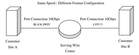
This example illustrates a same speed / different format circuit configuration whereby there is a 10Gbps WAN-PHY Port Connection between Customer Site A and the serving wire center and a 10Gbps OTU2 Port Connection between Customer Site B and the serving wire center. In this circuit example, both a 10Gbps WAN-PHY and a 10Gbps OTU2 Port Connection charge would apply.
