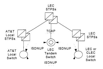
Figure 4. Interswitch TCAP Signaling for SS7 Network Interconnection [GTE opposes the use of figures and drawings]
