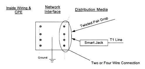
Figure 1 - Network Interface Device
