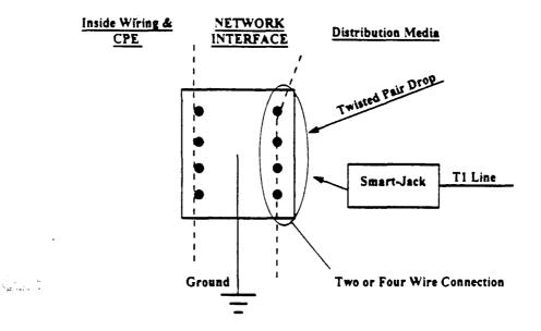
Figure 1 - Network Interface Device
