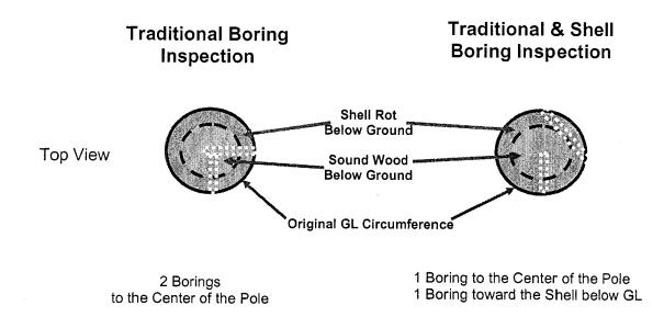
Osmose, which is the industry leader in wood pole inspections, considers this inspection procedure to be the best method available for poles that can't be excavated. Based on their experience, Osmose believes that this inspection method identifies priority poles with extensive below grade decay.
