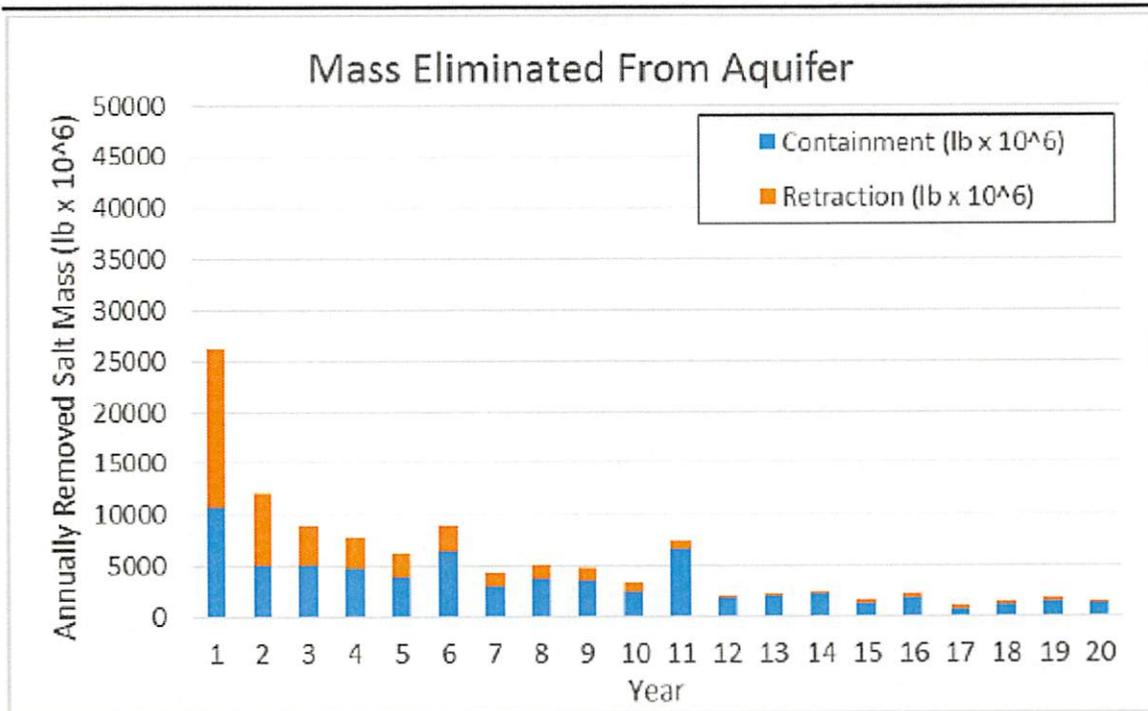
Demonstrative 27. Tetra Tech, 2016m, Figure 6: Containment and retraction mass reductions in the Biscayne Aquifer in each year of the model simulation (layers 1 through 11 evaluated).
