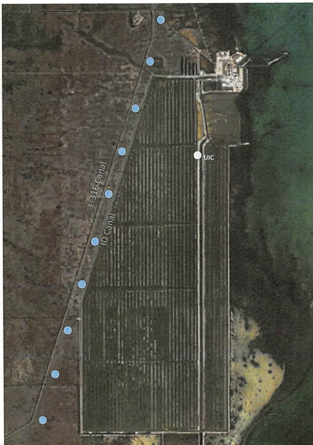
Figure 19. Configuration of extraction wells (blue dots) for Alternative 3D
