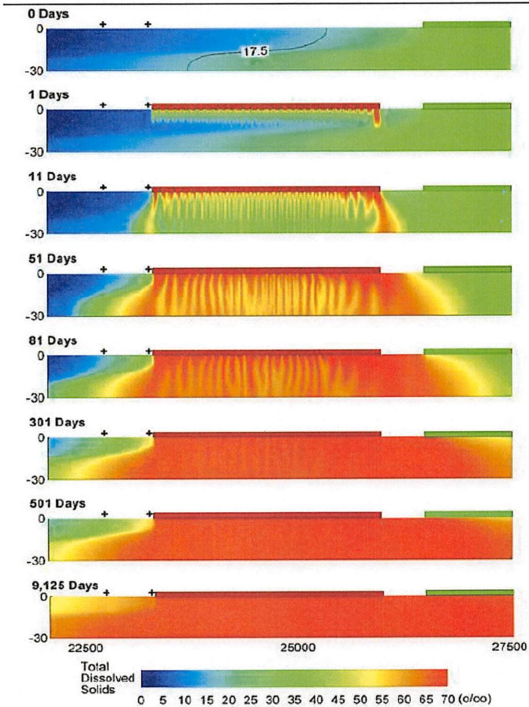
Demonstrative 16. Hughes et al (2009), Figure 4a: Simulated TDS concentrations for base simulation case A after specified days since cooling canal system construction.
