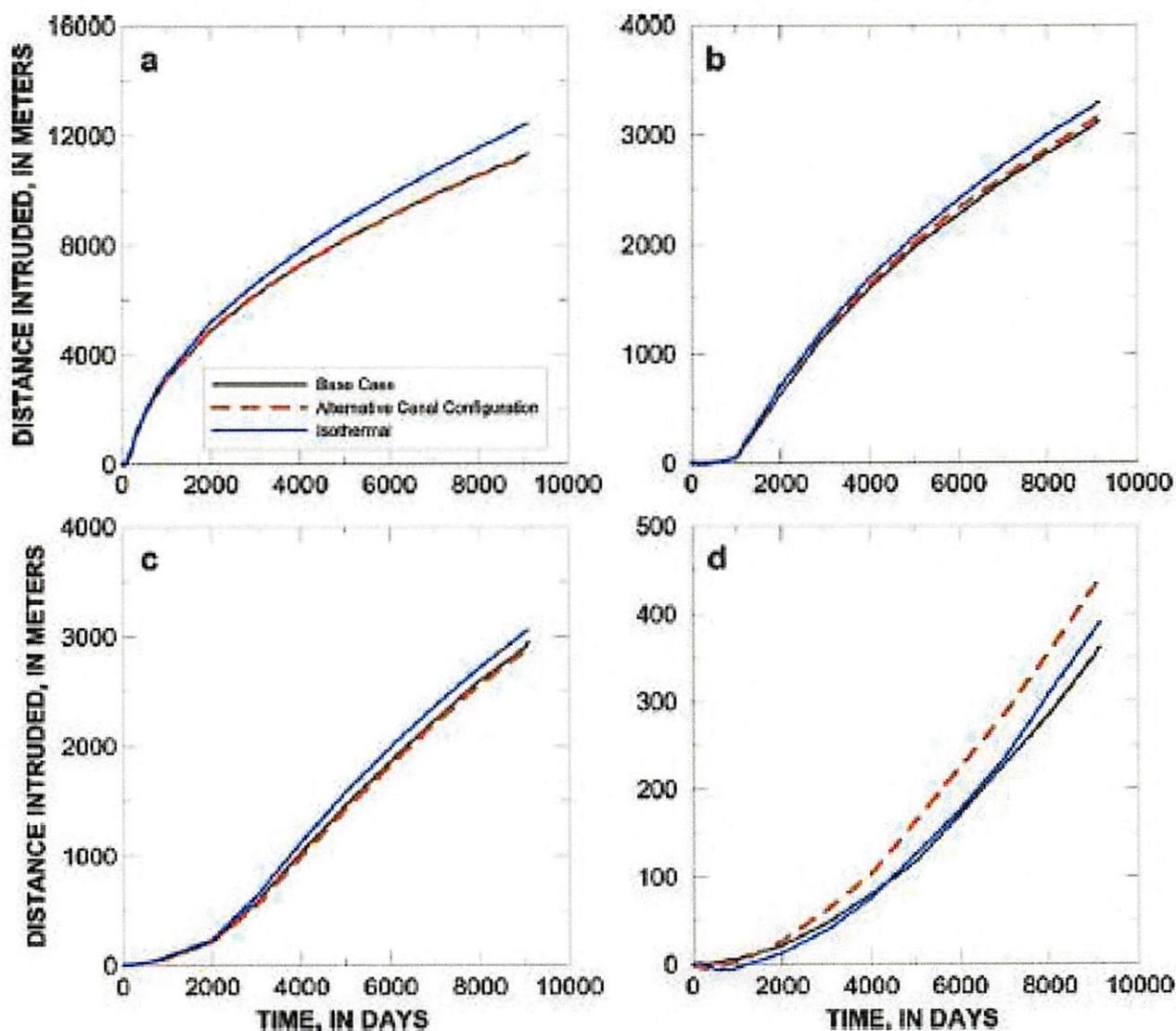
Demonstrative 17. Hughes et al (2009), Figure 7: Simulated movement of the 1% TDS concentration at the base of the aquifer
