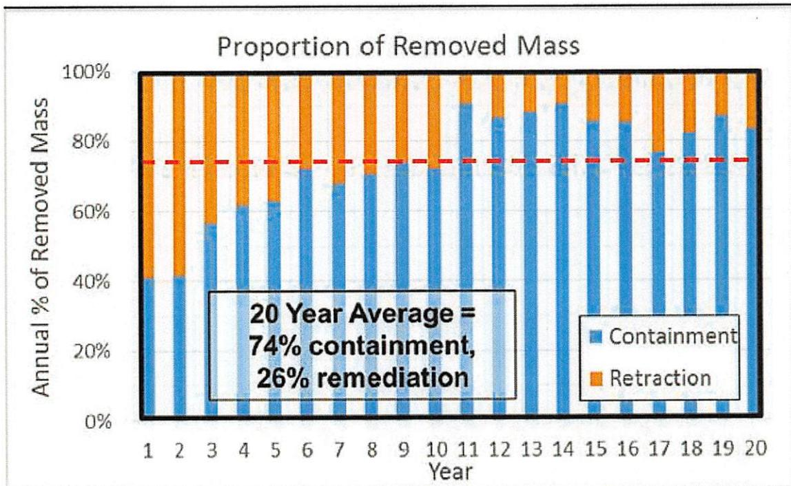
Demonstrative 28. Tetra Tech, 2016m, Figure 7: Proportions of containment and retraction mass reductions in Biscayne Aquifer in each year of the model simulation (layers 1 through 11 evaluated).
