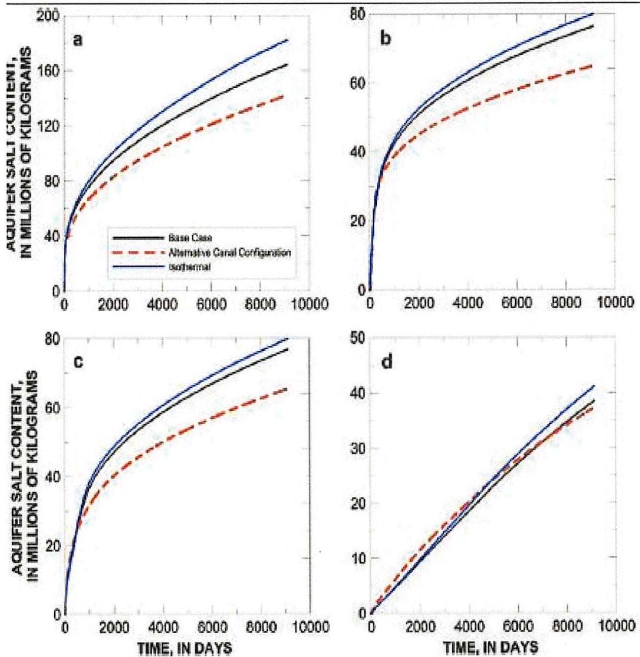
Demonstrative 18. Hughes et al (2009), Figure 6: Simulated increases in salt content of the aquifer as a result of CCS seepage.
