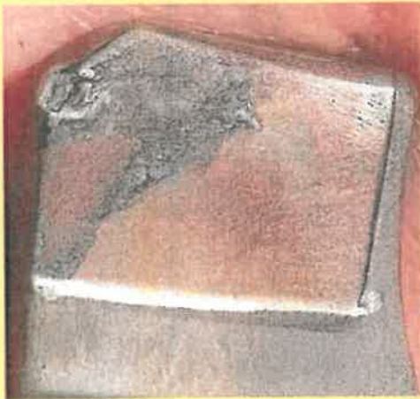
Figure 3 – Photo of an L-0 blade Z-Lock from Period 5 Showing Contact Surface Wear
