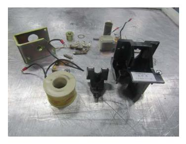
Disassembled Control Relay No issues were found with the control
