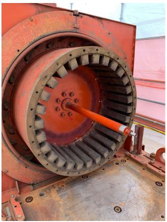
Fig. 8 PMG Pole Support w/ Magnets
