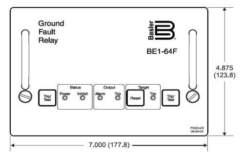
Basler field ground fault relay BE1-64F
