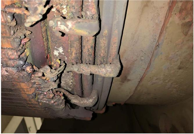
Fig. 7 PMG Stator Coil Connection Ring Failures
