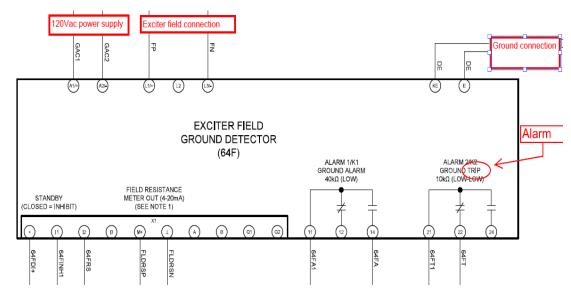
Exciter Field Ground Detector Module
