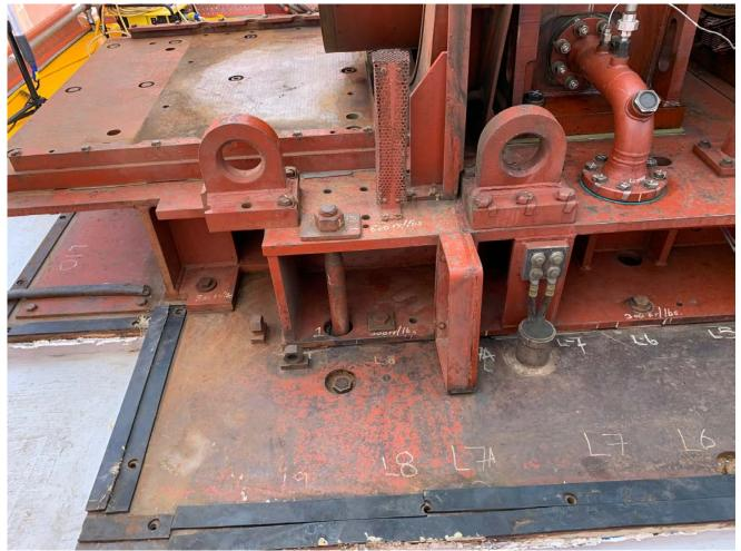
Fig. 13 Exciter Base to Housing Seal / Gasket Arrangement
