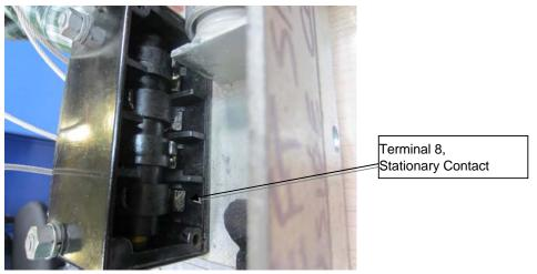
Left Side Switch - Switch Contact 4, Terminal 8
