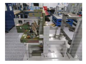
Breaker in Alignment Fixture
