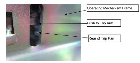
Operating Mechanism Inspection Hole
