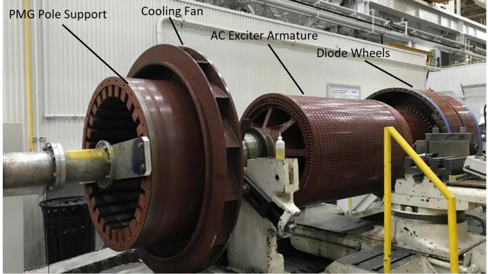
Fig 4 Exciter Rotating Element Removed
