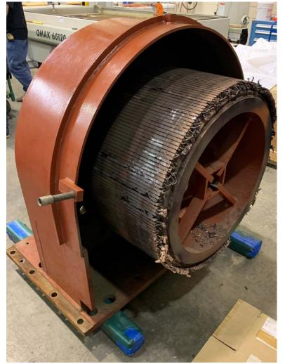
Fig. 5 U4 PMG Stator Removed
