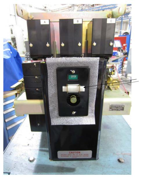
Refurbished DB-50 Breaker with Operating Mechanism Lock-Out Bar
