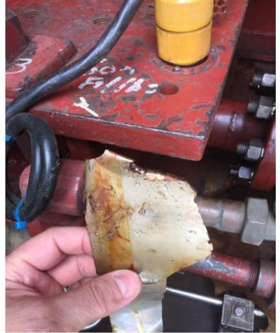
Fig. 12 Liberated Shim Stock Found in AC Exciter Section
