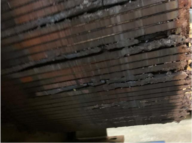
Fig. 6 PMG Stator Core – Coil Melt in Slots
