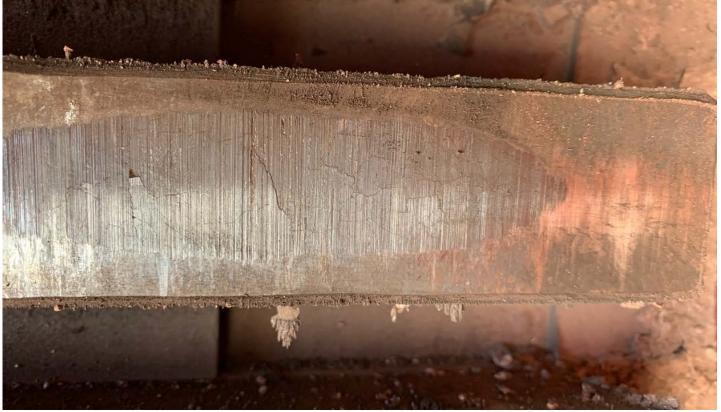
Fig. 10 PMG Magnet Cracking
