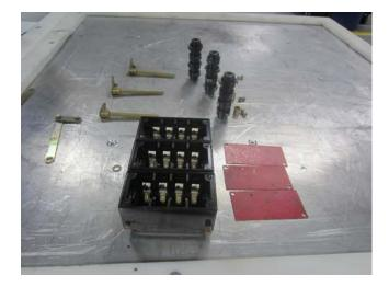
Disassembled Auxiliary Switches No issues were found with the auxiliary
