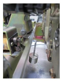
Additional Weight Added to the Operating Mechanism Trip Bar
