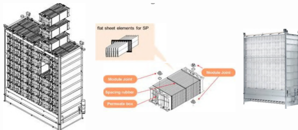
Figure 1. SP Series Unit Structure (left), Membrane Module Structure (center), and SP400 (right))
